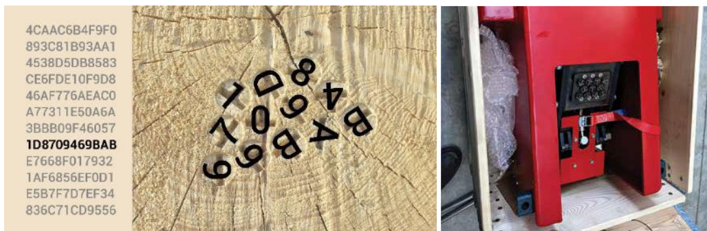
Figure 2: Punched mark and corresponding ID (left, source Otmotka.com) and punching tool for processor heads (right, source New Zealand Journal of Forestry 2023)
