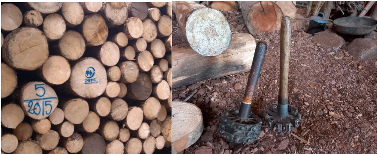
Figure 15: Log stack marked with colour (left) and brand hammers with variable code to identify the timber (right) (pictures: Picchi; right source: Musée des Métiers du Bois)
