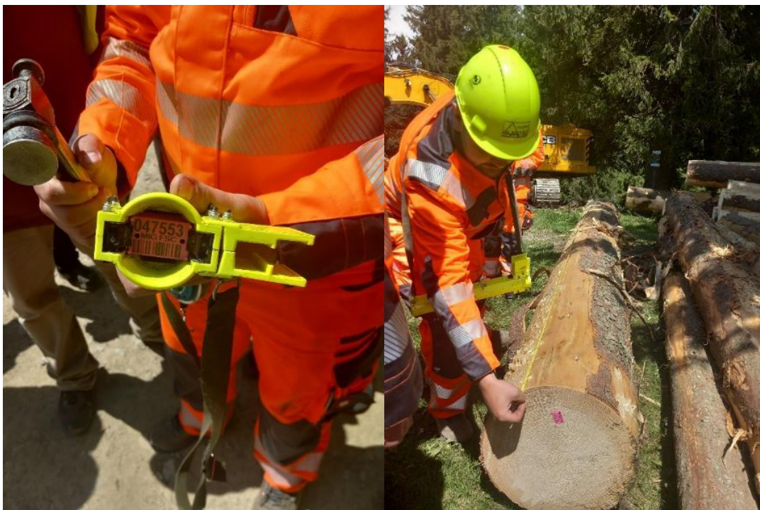
Figure 16: Hammer and magazine for plastic plaquettes (left) and operator measuring a log marked with a plaquette (right) (pictures: Picchi, CNR-IBE)
