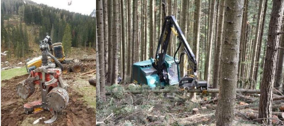
Figure 17: Single grip processor with feeding rollers (left) and stroke single grip processor delimiting a tree (right) (pictures: Picchi, CNR-IBE)
