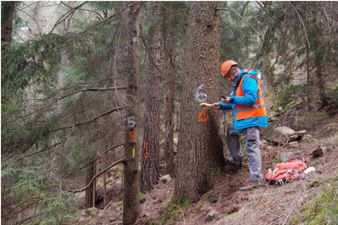
Figure 1: Operator reading RFID tags on standing trees with manual reader (source CNR-IBE)
