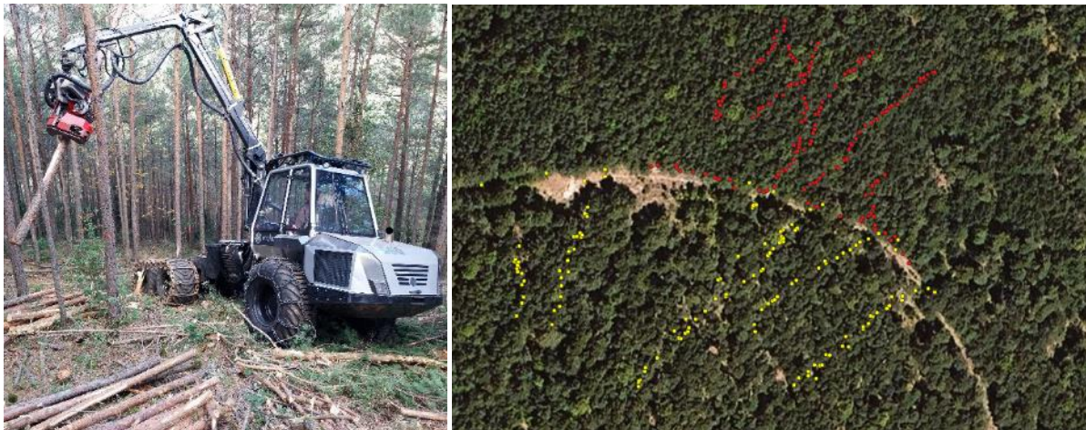
Figure 18: Forest harvester deployed to fell and process trees (left) map visualization of the georeferenced data reported in StanForD files regarding the position of the felled trees (right) (pictures: Picchi, CNR-IBE and Alcoverro, CTFC)
